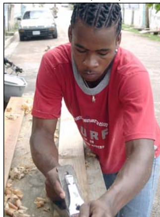
Learning how to operate traditional hand tools, Trainee Calvin Hall uses a donated hand planer at 3A Lower Harbour Street.
