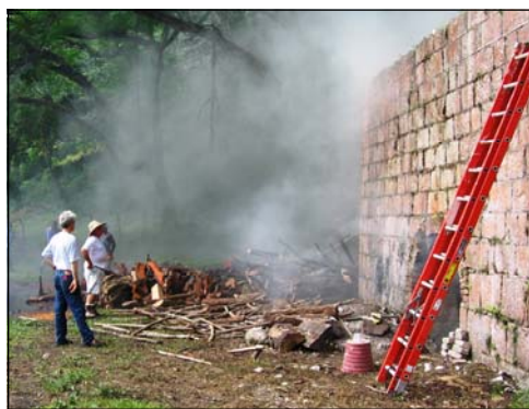
Dr. Ed Chappell of Colonial Williamsburg and Jeffery Price of Virginia Lime Works watch on as an 18th century limekiln was fired at Good Hope Country House in order to make quicklime used in the process of preparing historic-grade lime putty.
